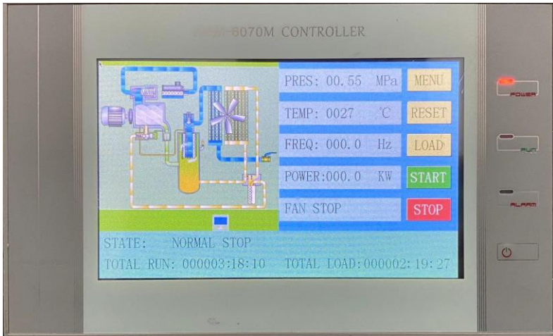
Figure 4-15 Main working interface of the Plot controller
