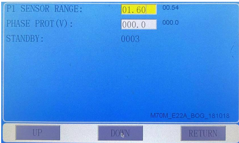
Figure 4-20 Calibration parameter setting interface
